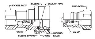
Series HK Couplings are designed for general purpose hydraulic service. Some are suitable for use with various liquids, chemicals, steam, gases and vacuum. Series HK couplings conform to the dimensional requirements of ISO 7241-1 Series B. Body sizes range from 1/8" to 2-1/2".
