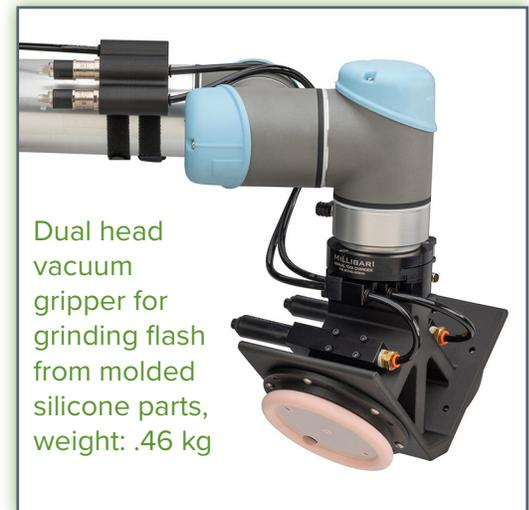
Dual head vacuum gripper for grinding flash from molded silicone parts, weight: .46 kg
