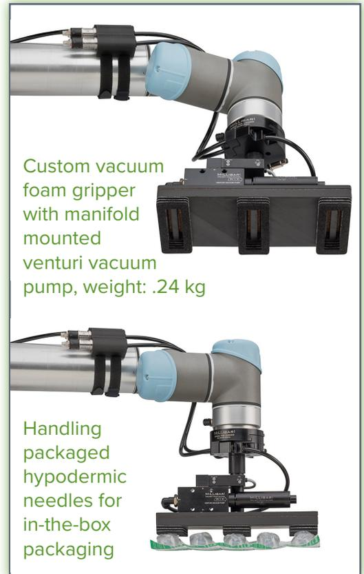
Custom vacuum foam gripper with manifold mounted venturi vacuum pump, weight: .24 kg
