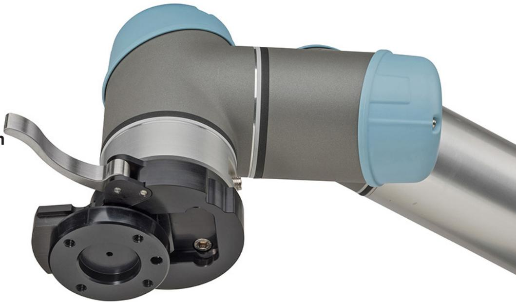
The Low Profile tool changer adds just 21mm (.83") to the height of the wrist of the robot and, weighing just .3 kg, has a minimal impact on payload.
